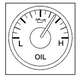
The oil pressure indicator tells you if you have the correct oil pressure in your engine to operate your vehicle.
